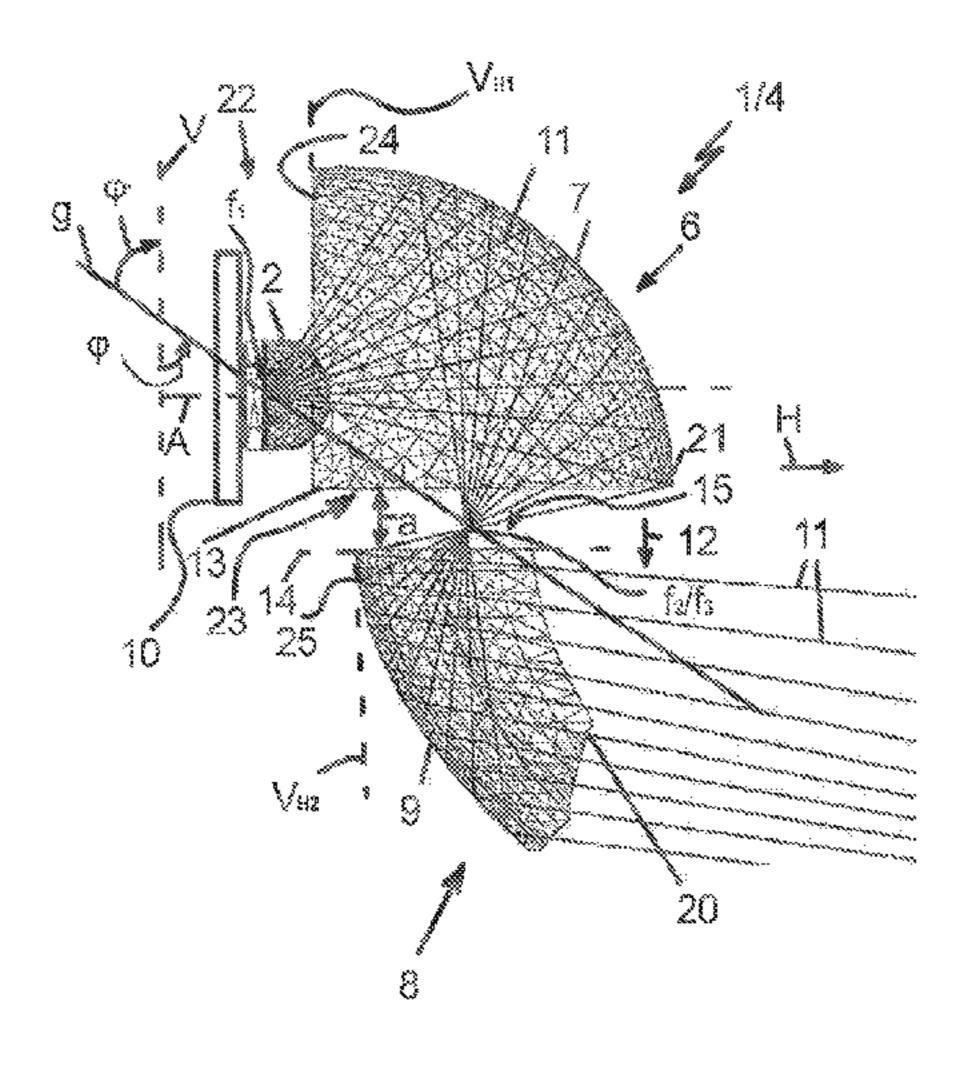
first opening portion and facing towards the second reflector. The reflector surface of the second reflector has free-form parts such that light striking the reflector surface of the second reflector is reflected in such a way that a light distribution having a predetermined light/dark boundary is produced.
