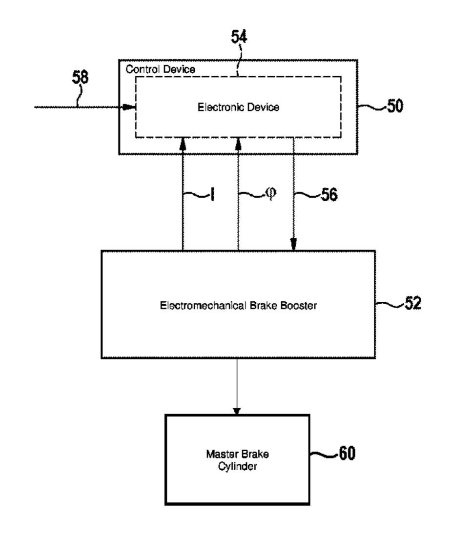
to the motor. The electronics unit defines a maximum target variable with respect to a maximum target rotational speed of the motor, taking into account a current intensity of a motor current of the motor and a current angle of rotation of a rotor of the motor, and defines the target variable with respect to the target rotational speed of the motor of the electromechanical brake booster to be at the most equal to the defined maximum target variable.
