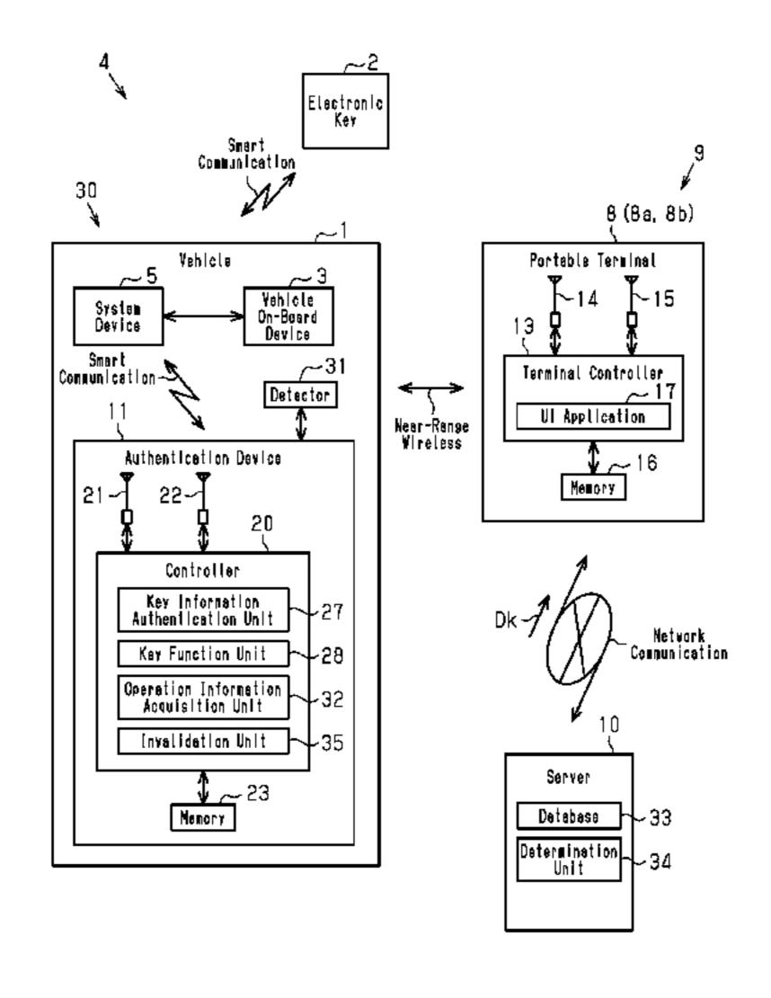
performs a predetermined action when the vehicle operation is determined as being abnormal. The determination unit uses the wireless authentication functionality to execute at least part of a series of processes of the abnormality determination and the predetermined action.
