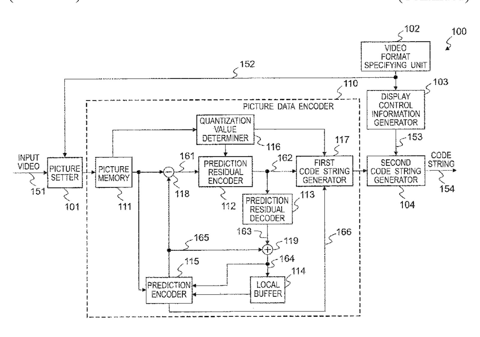
each other, and encoding a picture to be encoded which is the frame or the field with reference to a picture previously encoded before encoding the picture to be encoded. In the encoding, the video is encoded with a syntax structure which is not dependent on the video format, the video format information is encoded in a header of a sequence which is a unit of the video, and the encoded bit stream is generated.
