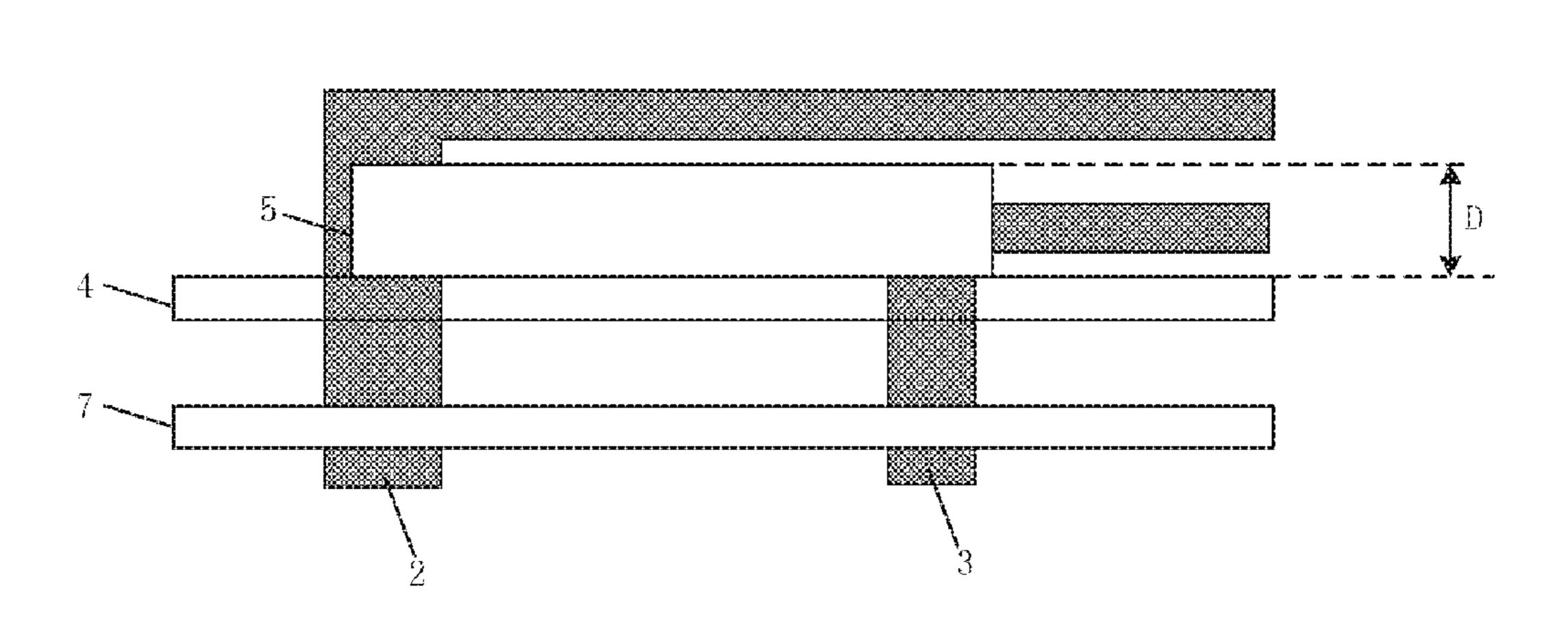
power supply line, the negative power supply line and the first dam are in the peripheral region, and the first dam is arranged around the display region. At least in a corresponding region between the positive power supply line and the negative power supply line, a protruding structure is on a side of the first dam proximal to the display region.
