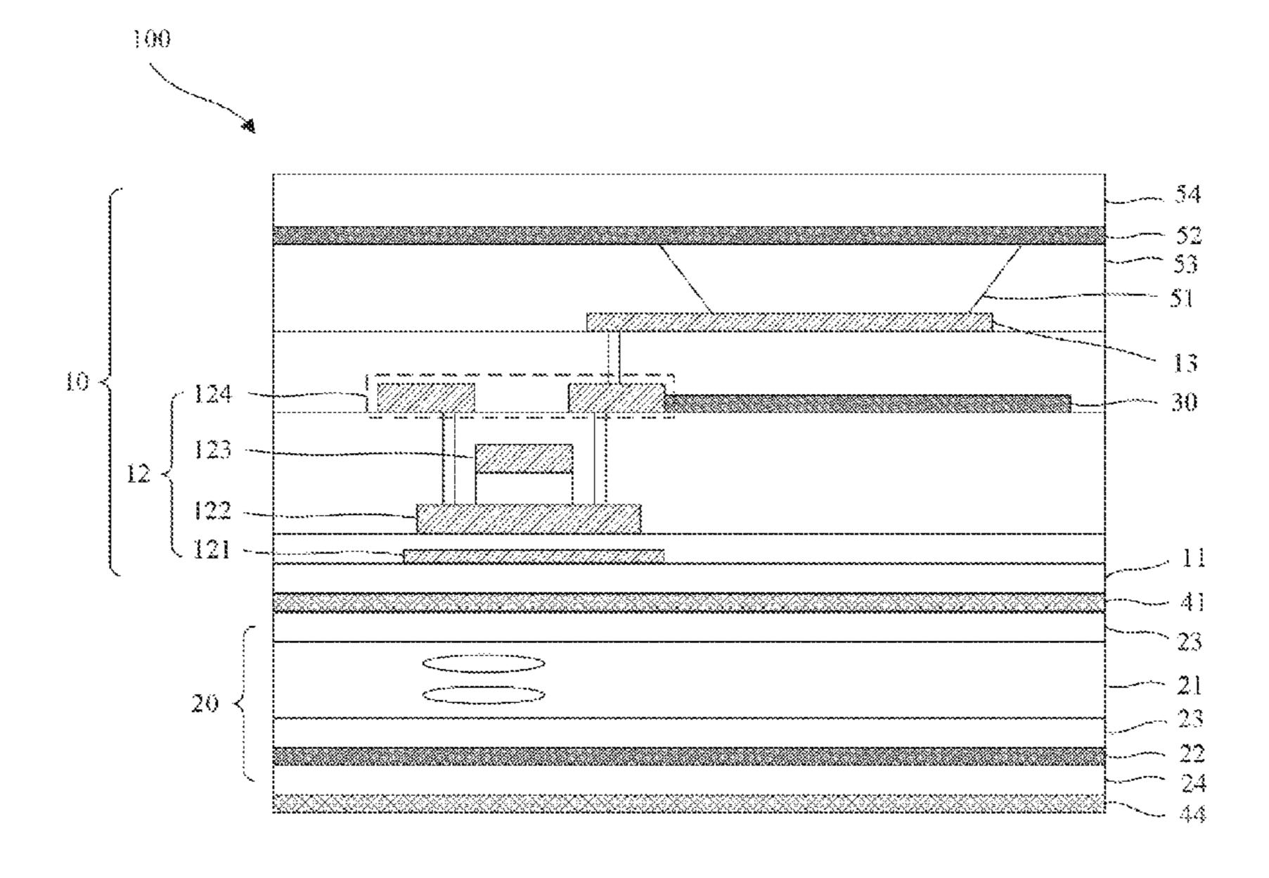
on the first substrate, and the driving circuit layer allows the first sub-display panel or/and the second sub-display panel to transmit light.
