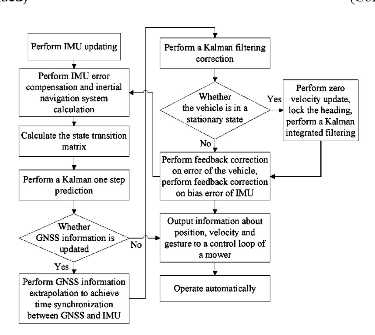
parameter of the mobile vehicle based on the error estimation value of the motion state; and controlling an operation route of the mobile vehicle based on corrected navigation information.
