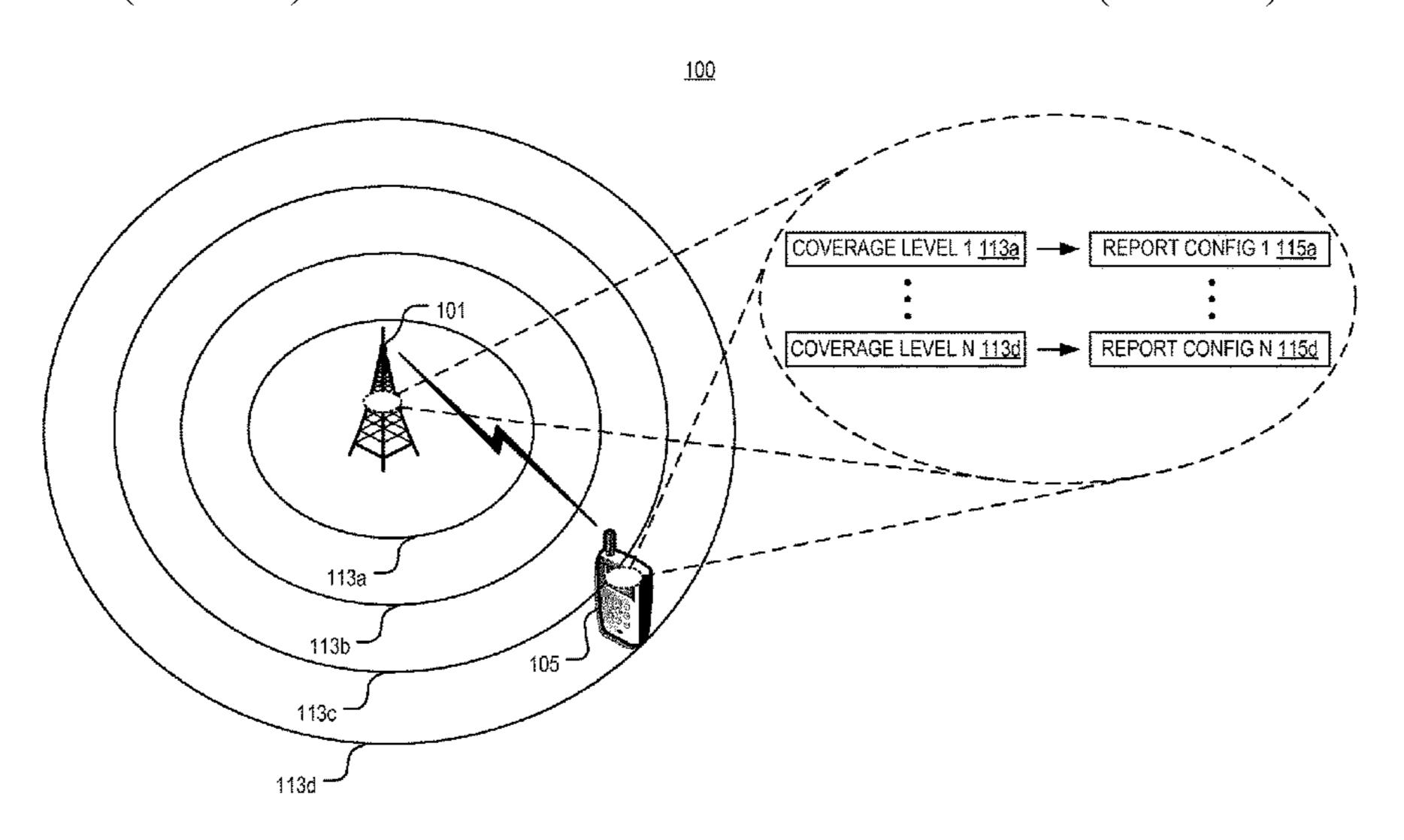
age levels of the wireless device, the reporting configuration associated with the coverage level indicated by the obtained information. Also, the method includes reporting (511) a measurement result using the determined reporting configuration.
