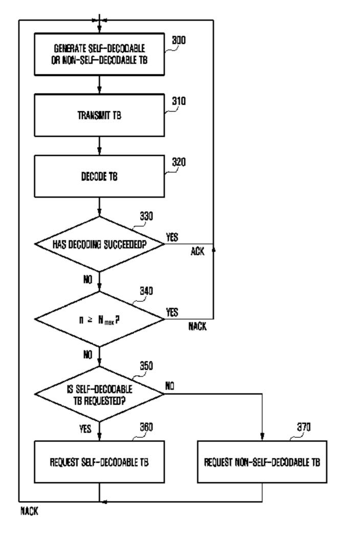
step of transmitting a data packet to a receiver, receiving hybrid ARQ (HARQ) feedback information based on a decoded result of the data packet, generating a data packet to be re-transmitted on the basis of the HARQ feedback information, and transmitting, to the receiver, the data packet to be re-transmitted, wherein the HARQ feedback information can include acknowledgment (ACK) or negative-acknowledgment (NACK) and information including a HARQ status of the data packet.
