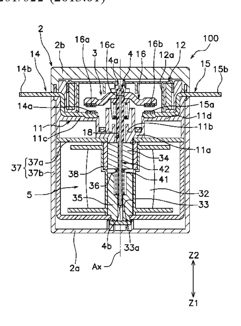
contact portion configured to contact the movable iron core, and an insulating portion made from an insulating material and configured to insulate the movable contact piece and the movable iron core from each other.
