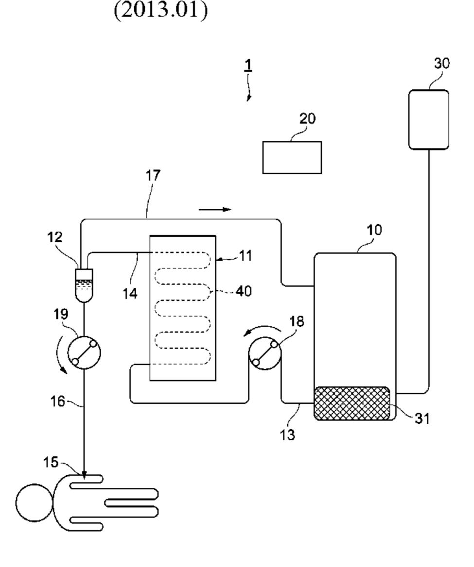
On the heat plate, a heater in a predetermined pattern corresponding to the warming flow path is disposed. The heater is disposed such that an amount of heat generation toward the warming flow path decreases in stages from an upstream side toward a downstream side in the warming flow path and that a decrease rate of the amount of heat generation at each of the stages decreases from the upstream side toward the downstream side.
