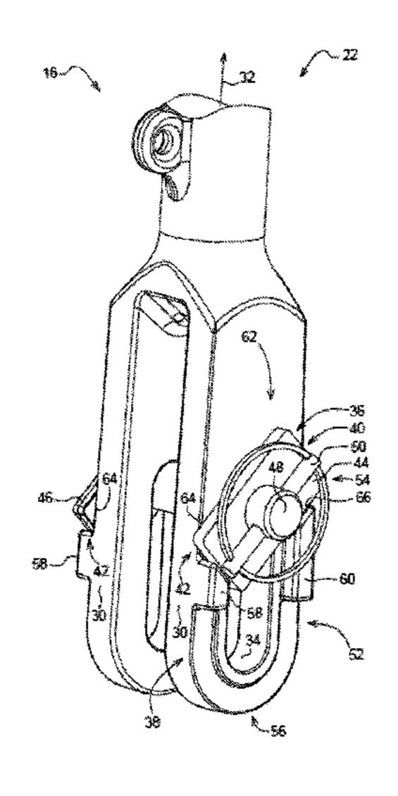
of the link arm along the elongated hole is blocked when the shaped feature is received in one of the locking regions.
