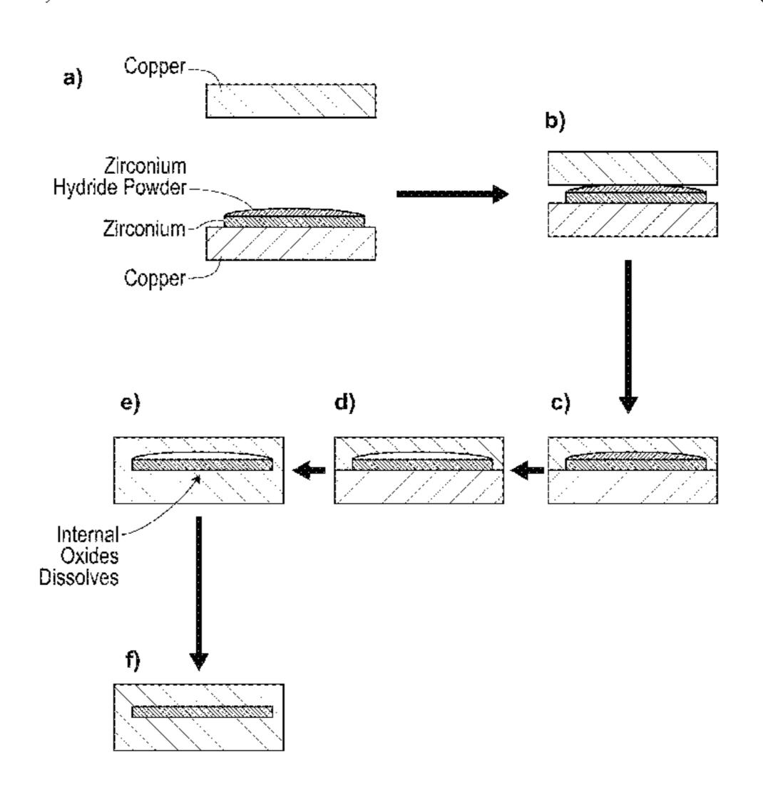
assembly. Load is applied to the assembly and the assembly is heated. The shell metal deforms around the article and the metal hydride and forms a gas proof seal. The metal hydride thermally decomposes to form hydrogen gas. At least a portion of the hydrogen gas dissociates and moves as monoatomic hydrogen into the article. The metal alloy can be a zirconium metal alloy, the metal hydride can be a zirconium metal hydride, and the shell metal can be substantially copper.
