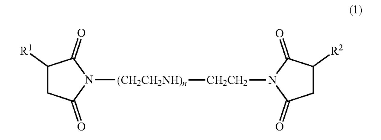
wherein in the general formula (1), R<sup>1</sup> and R<sup>2</sup> each independently represent a hydrogen atom or a C1-36 linear or branched chain alkyl or alkenyl group, and at least one of R<sup>1</sup> and R<sup>2</sup> is a C8-36 linear or branched chain alkyl or alkenyl group, and n represents an integer of 1 to 10.
