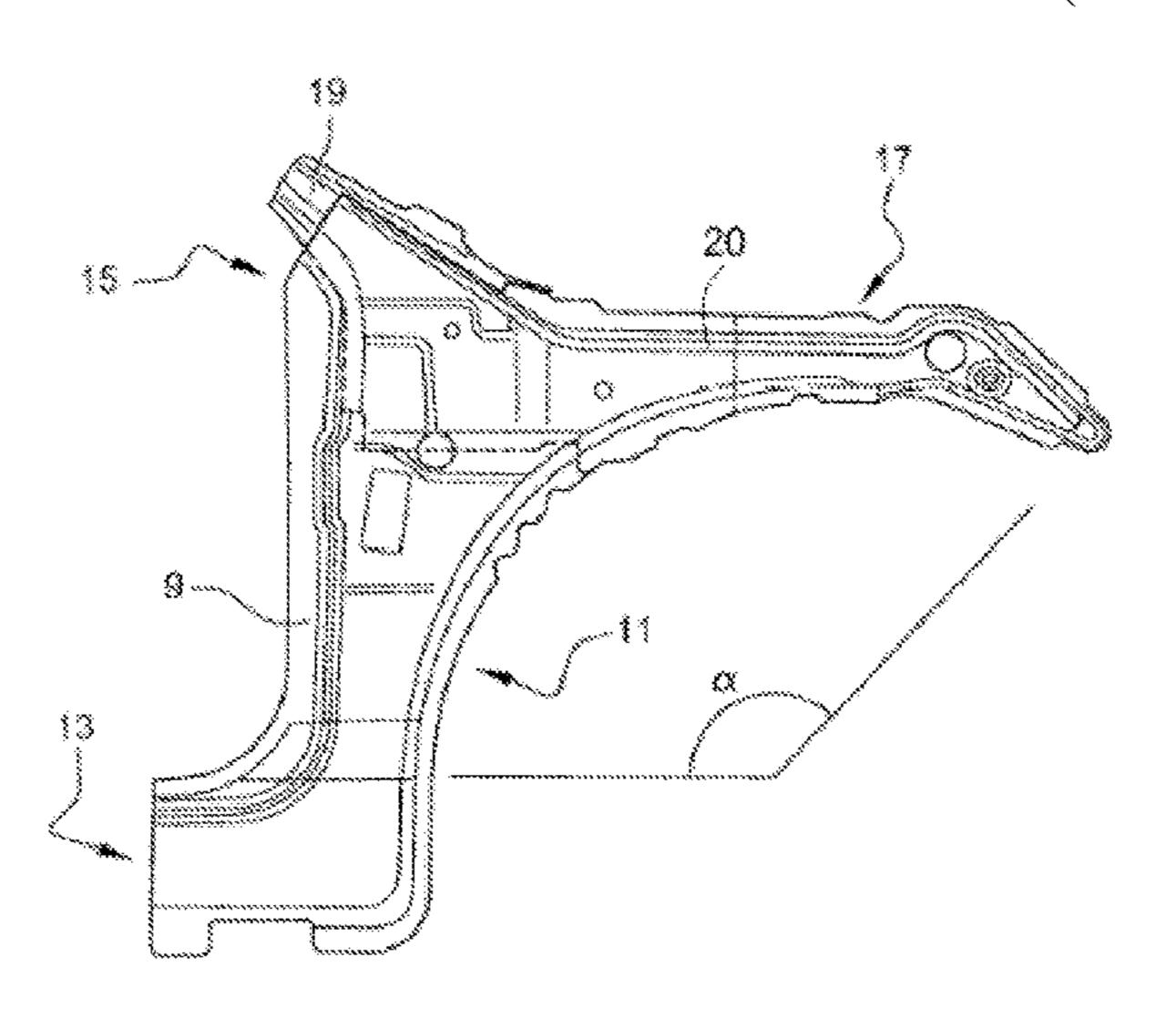
body (11) and said front extension (17) form a single part. The invention also relates to the methods for producing such a front hinge pillar (9).
