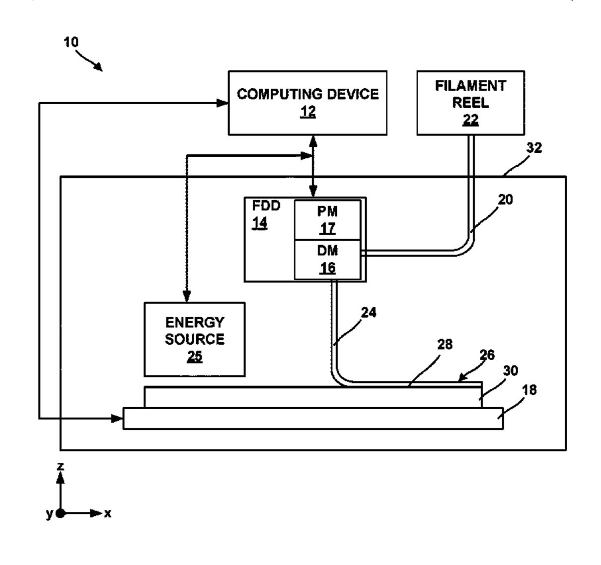
fabricated component to leave an unsintered component; and sintering the unsintered component to join particles of the SMA and form an SMA component.
