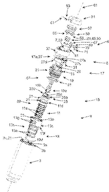
tive modes, the actuating assembly (17) being manually operated and having at least one actuating component (17a), such an actuating ring (27), for example, being provided about a peripheral surface of the containment vessel (1).
