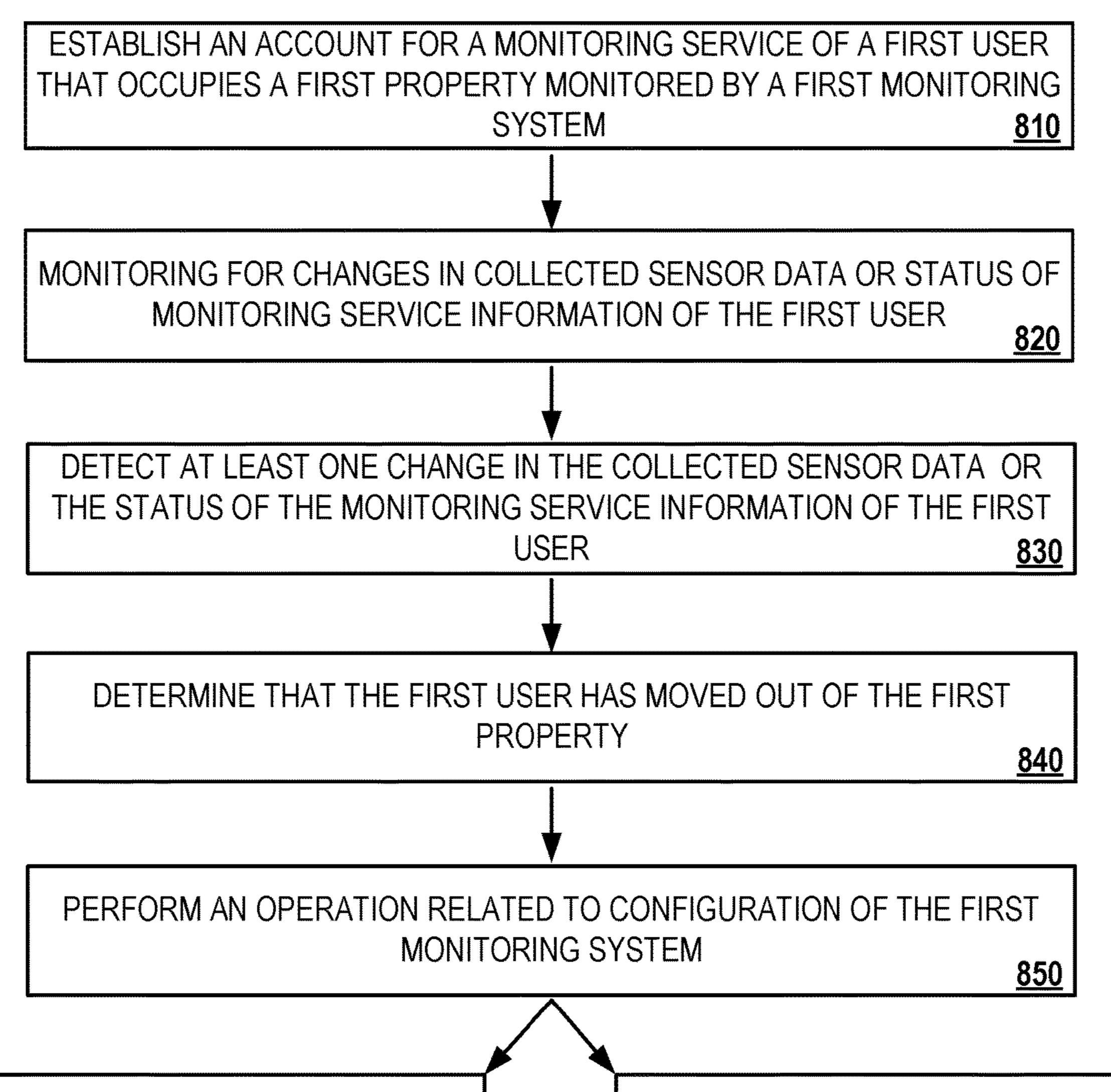
USE THE FIRST CONFIGURATION INFORMATION FOR THE FIRST MONITORING SYSTEM TO CONFIGURE THE FIRST MONITORING SYSTEM FOR A SECOND USER THAT HAS MOVED INTO THE FIRST PROPERTY 860A
