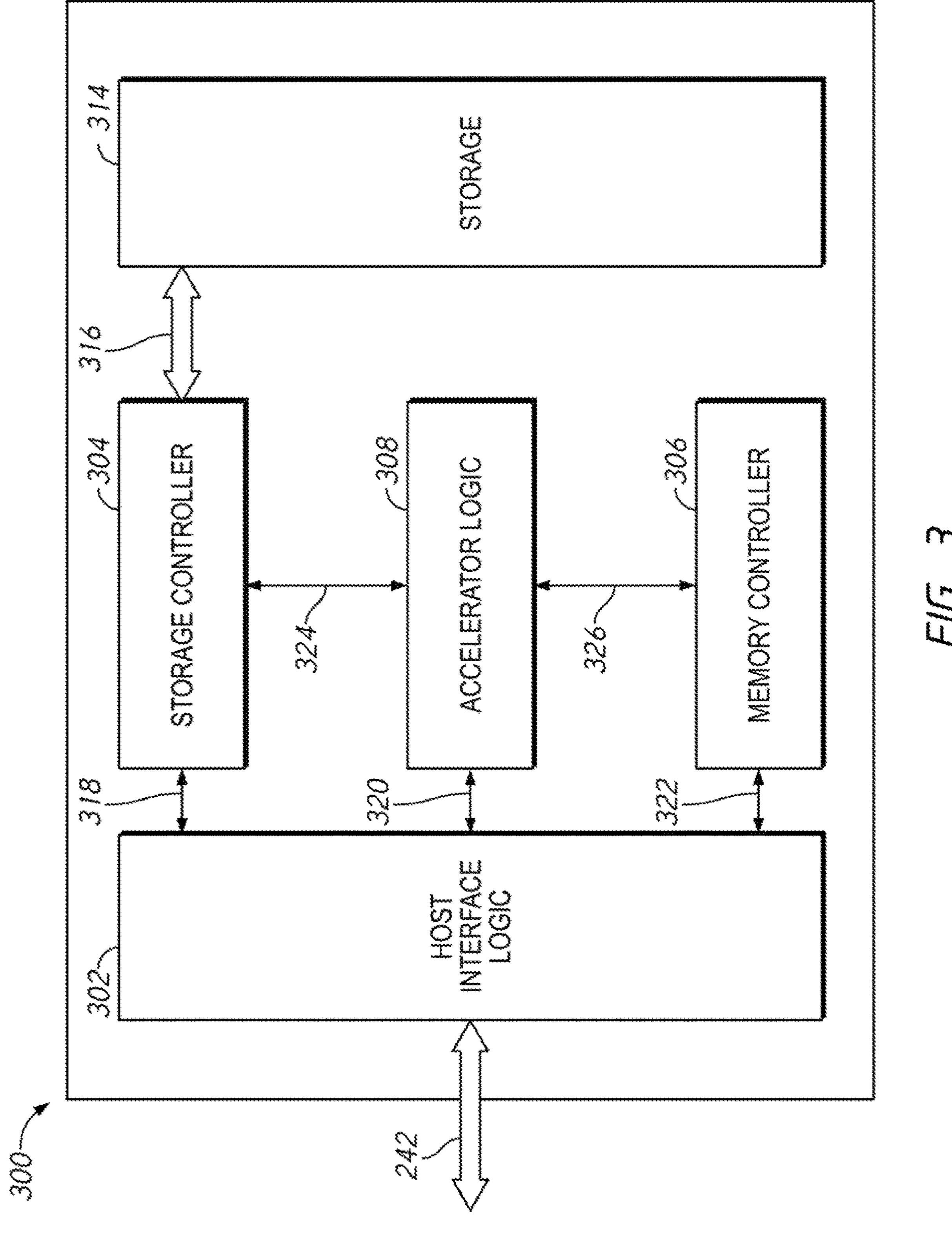
ACCESS DATA RESIDING ON THE STORAGE COMPONENT VIA AN ACCELERATOR STORAGE PATH PROVIDING AN INTERFACE BETWEEN THE ACCELERATOR AND A STORAGE CONTROLLER MANAGING THE STORAGE COMPONENT
