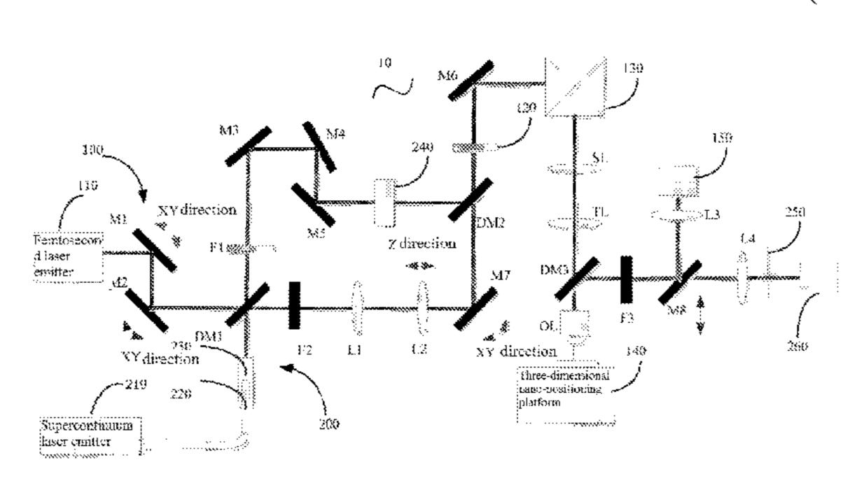
types of light spots generated by an excitation light and a depletion light after being focused by an objective lens accurately coincide in a three-dimensional distribution, thereby providing a powerful tool for cutting-edge biomedical research.
