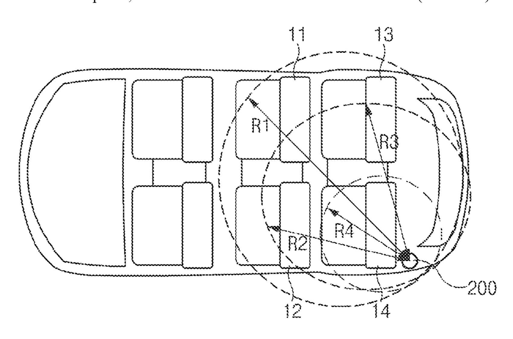
each distance and information associated with strength of a radar signal according to the reflection characteristics of the medium.
