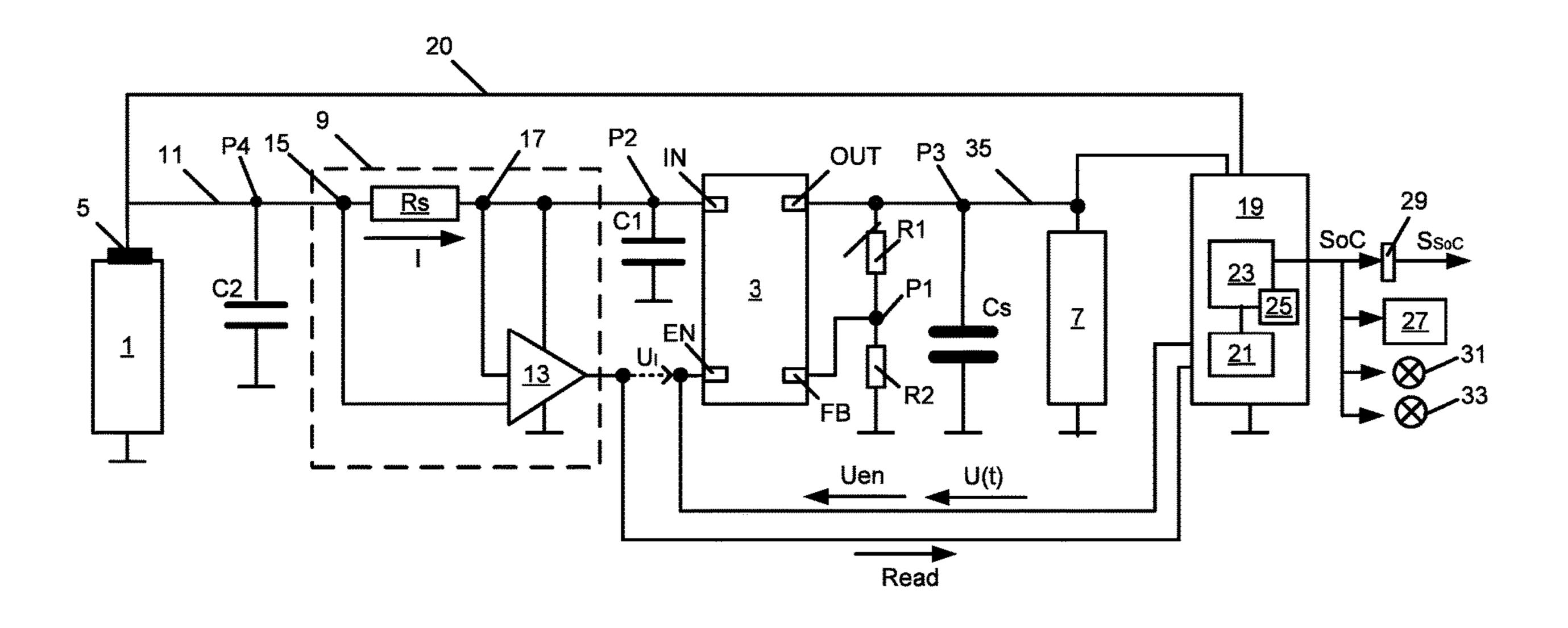
least once determining and providing a state of charge of the battery determined based on a duration of at least one first time interval during which the voltage converter was enabled during one of the duty cycles and a previously determined dependency of the durations on the state of charge of the battery.
