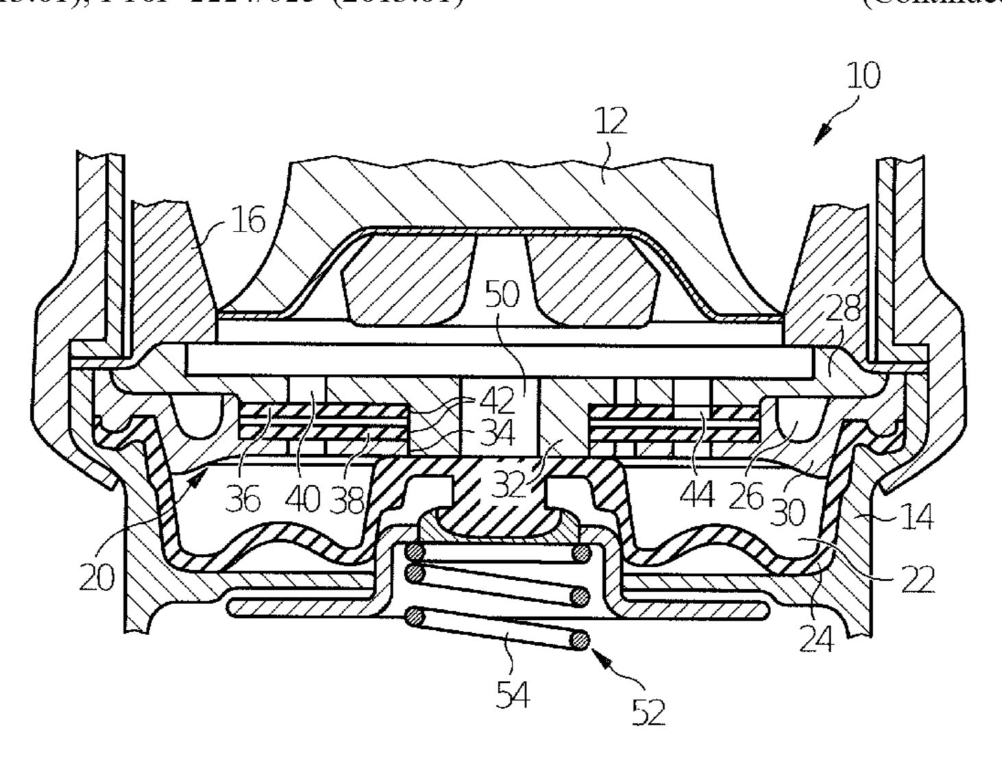
membrane are arranged, and wherein one of the membranes has at least one through-hole.
