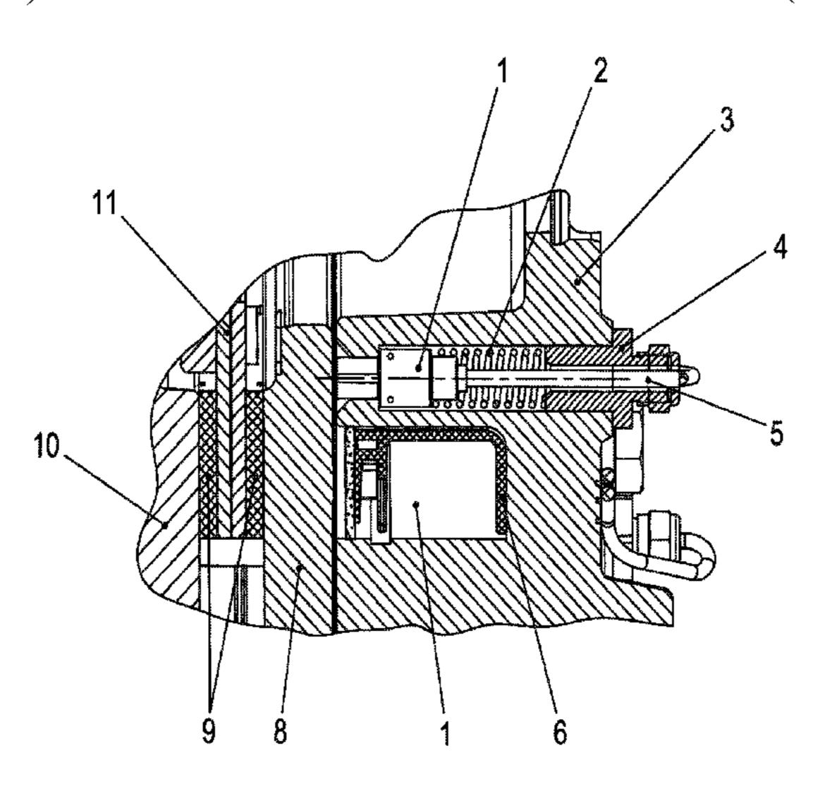
side and on the screwed cable gland on the other, and the sensor housing is pressed against a step of the bore, in particular by the spring part.
