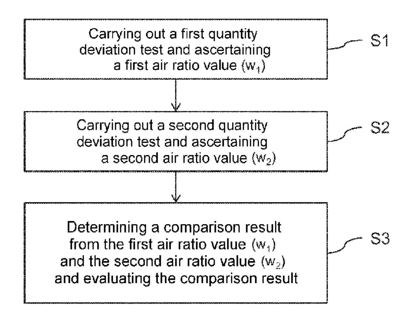
chambers of the internal combustion engine, wherein in the second quantity deviation test, a load control is carried out by the throttle valve; and lastly c) determining a comparison result from the first air ratio value and the second air ratio value, the presence of a fault in the intake tract of the internal combustion engine being detectable using the comparison result.
