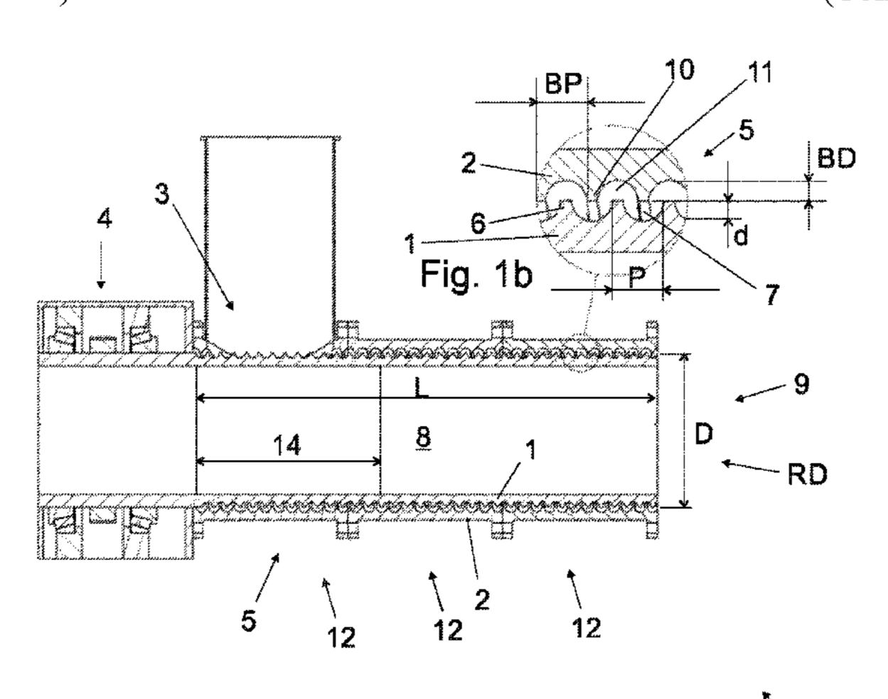
compris-ing—a drive system (4) for the rotation of the rotor member (1) in the barrel (2). The relation of the depth (d) to the diame-ter (D) of the rotor member, i.e. d:D, is not more than 1:20, and the relation of the pitch (P) of the rotor member to the di-ameter (D) of the rotor member, i.e. P:D, is not more than 1:4.
