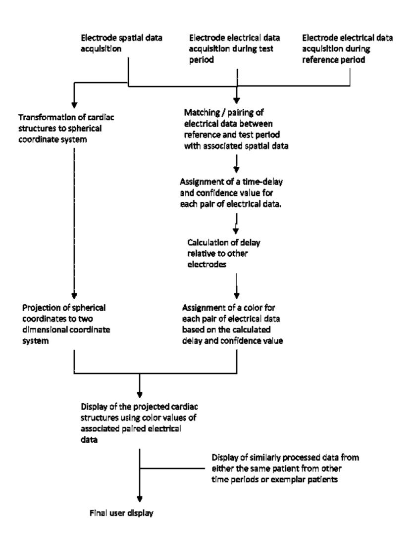
of electrograms for each of the plurality of spatial locations, and deriving a time delay for each spatial location by calculating the time delay between the electrograms of the pair of matched electrograms for that spatial location.
