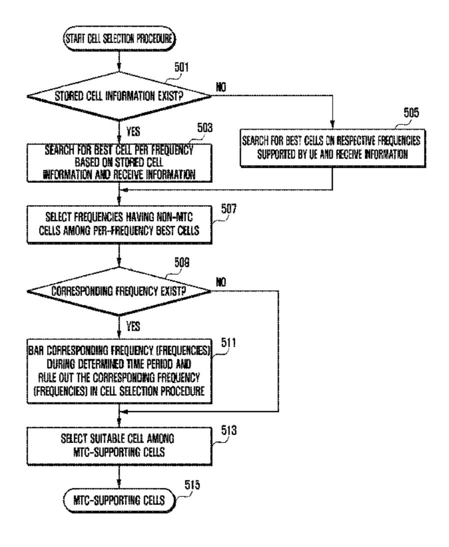
scanning a frequency used in communication with the base station during a determined period.
