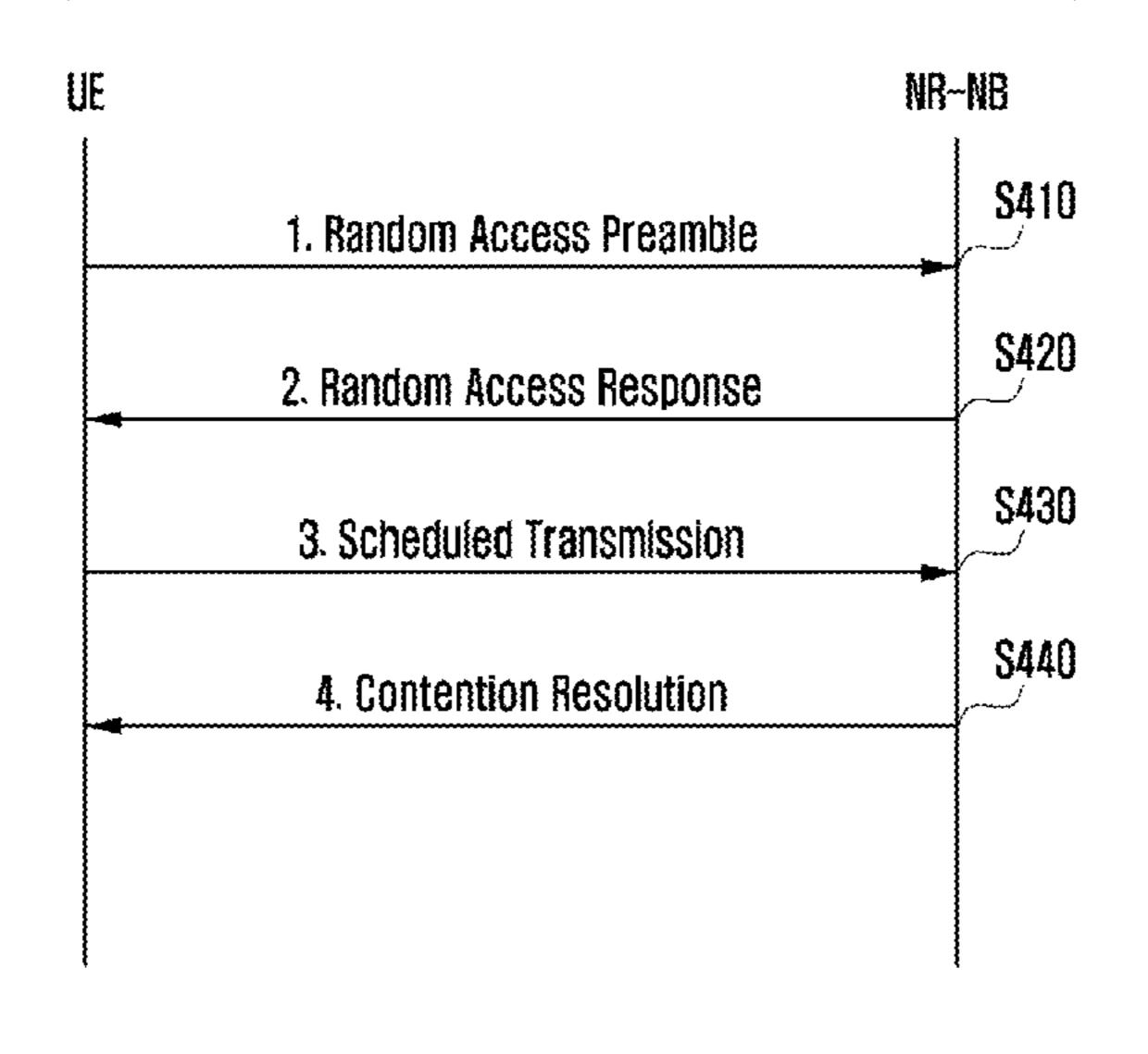
base station, a scheduled transmission message over a third bandwidth selected among the plurality of channel bandwidths of the UE.
