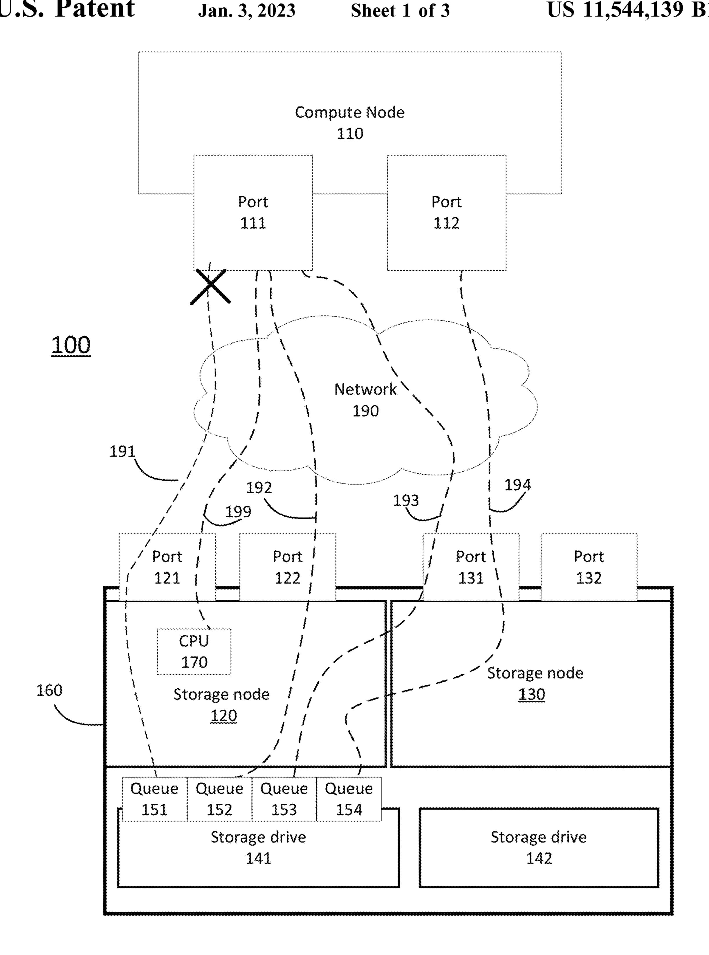
Sending over a path a remote direct write request associated with a certain address range. The path is formed between a compute node of a storage system to a storage drive of the storage system. 210
