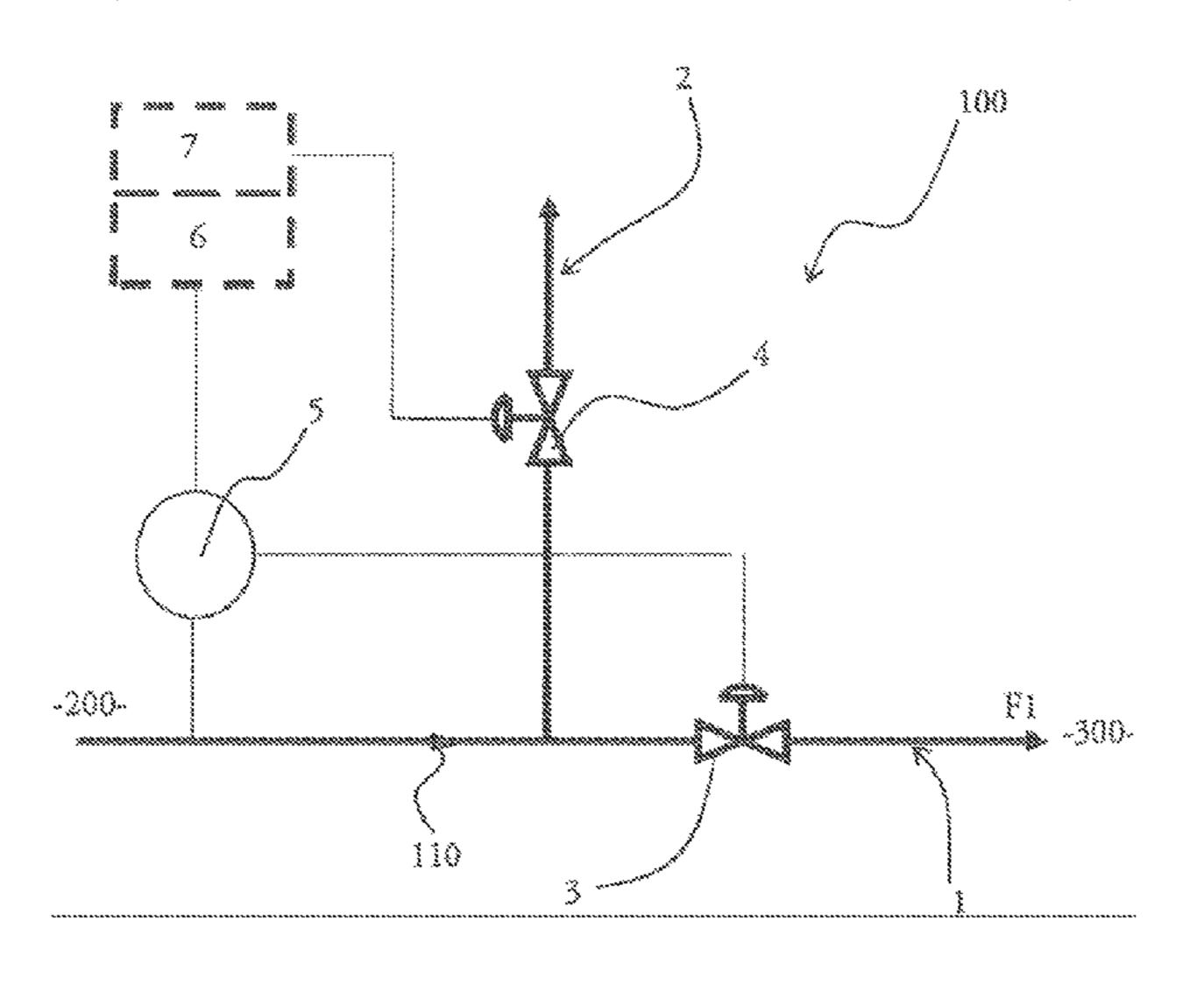
parameter and means configured to control the partial gradual opening or closing of the discharge valve depending on the result of the comparison of said sliding threshold value with an instantaneous value of the characteristic parameter, in order to improve reliability of the industrial facility.
