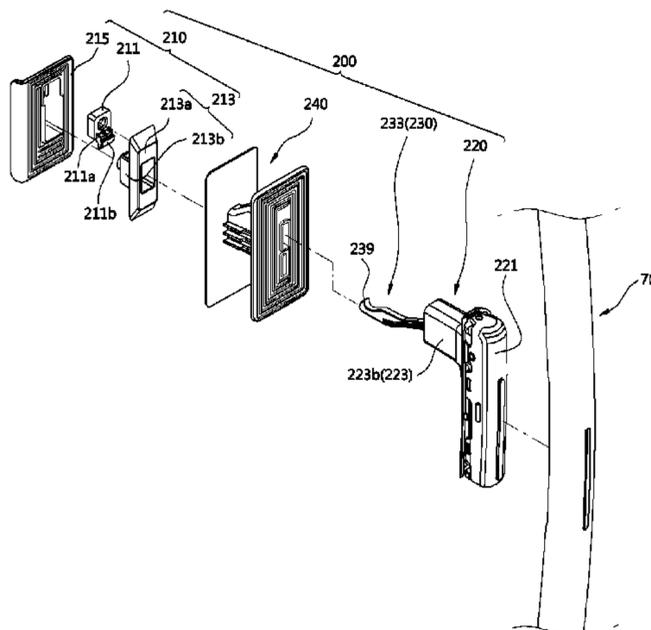
device allowing the second door to be fixed and released to/from the first door.
