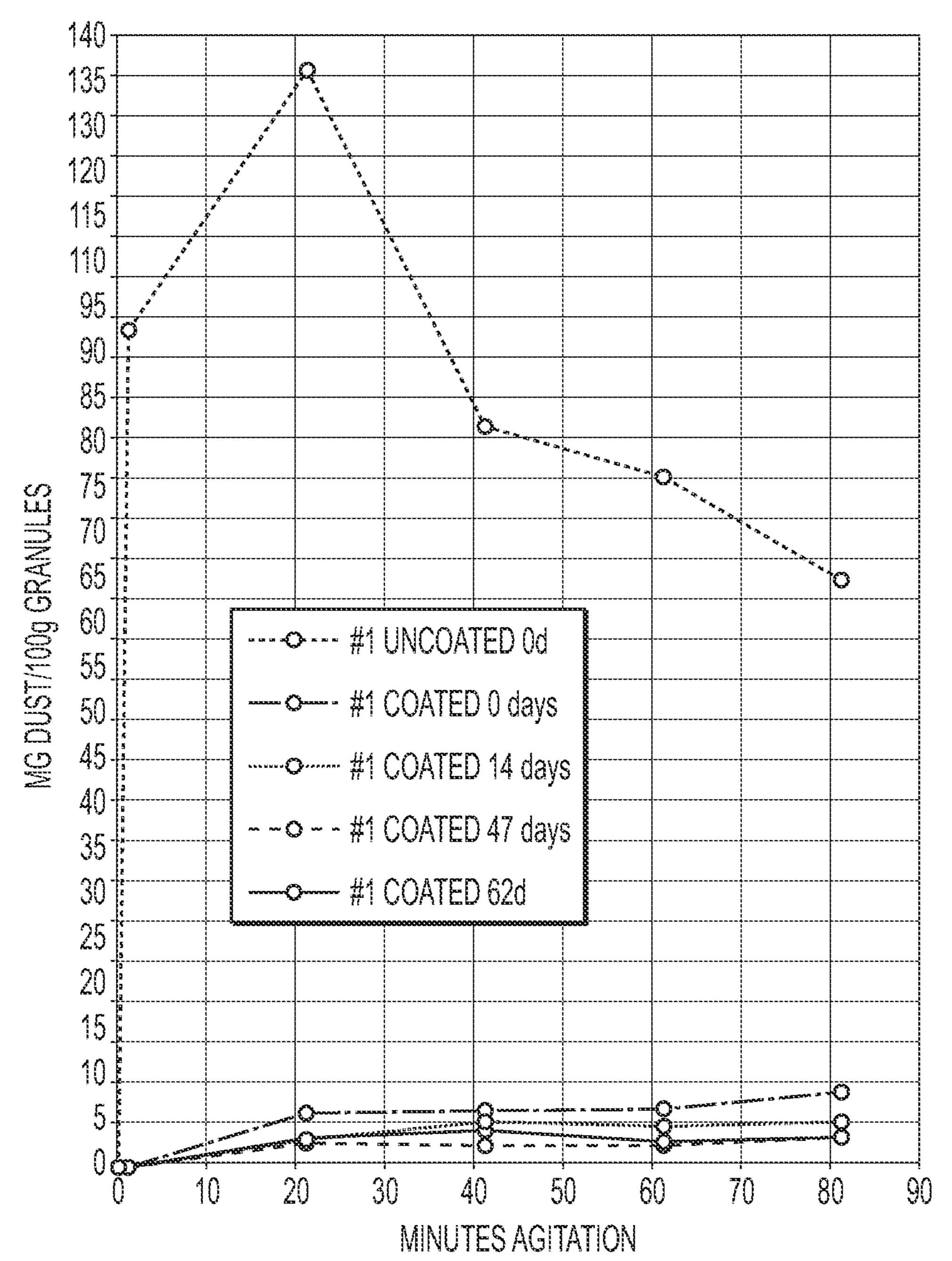
\* HEUBACH DUSTMETER TYPE I RUN W 200g SAMPLES @ 30 RPM & 20L/min AIRFLOW \* ANY DUST COLLECTED IN INITIAL 1\* CONSIDERED TREE DUST
