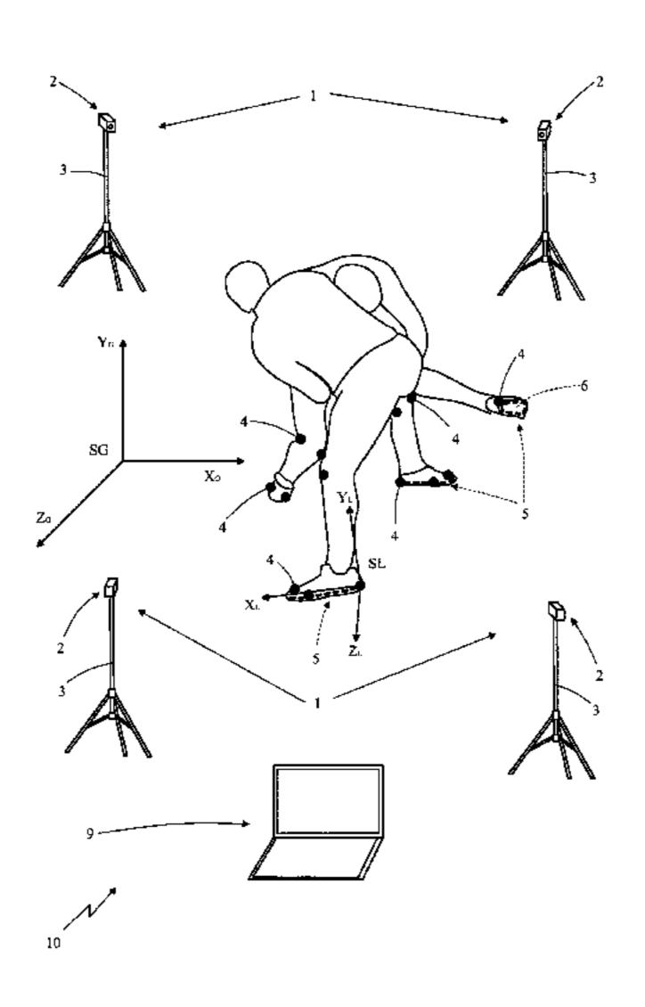
parameters, the coordinates of the center of pressure (COP) of the foot and of the constraining reaction force (FV) acting on the foot; a step for calculating a force arm (BF) given by the distance between the center of pressure (COP) and a reference point (PR) of the knee; a step for calculating a biomechanical parameter indicative of the valgus moment, derived from the vector product (PV) of the force arm (BF) and the constraining reaction force (FV).
