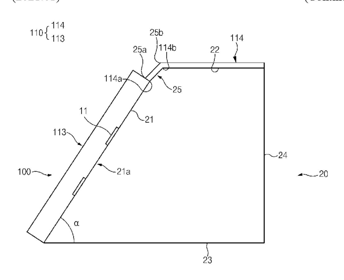
battery case. The body is pressed to discharge a gas accommodated in the accommodation part through the gas pocket part in the battery case. This method allows easy discharging of internal gas while reducing discharge of the electrolyte with the gas.
