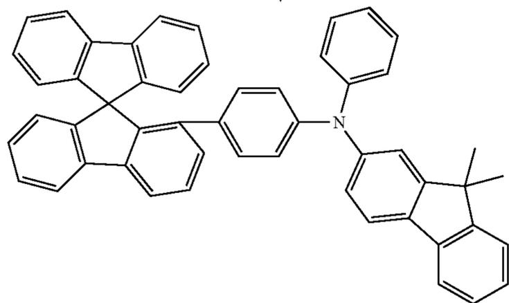
Example 3a: Synthesis of phenyl-2-(9,9'-dimethyl-fluorenyl)-1-spiro-9,9'-bifluorenylamine
