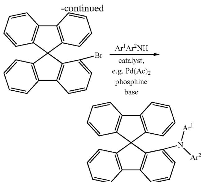
Analogously to the classical spiro synthesis shown above, the corresponding spirobifluorene derivatives which are halogenated in the 3- or 4-position can be synthesised by employing the corresponding 3- or 4-halogen-substituted fluorenone as starting material. Likewise, corresponding substituted structures can also be synthesised entirely analogously.
