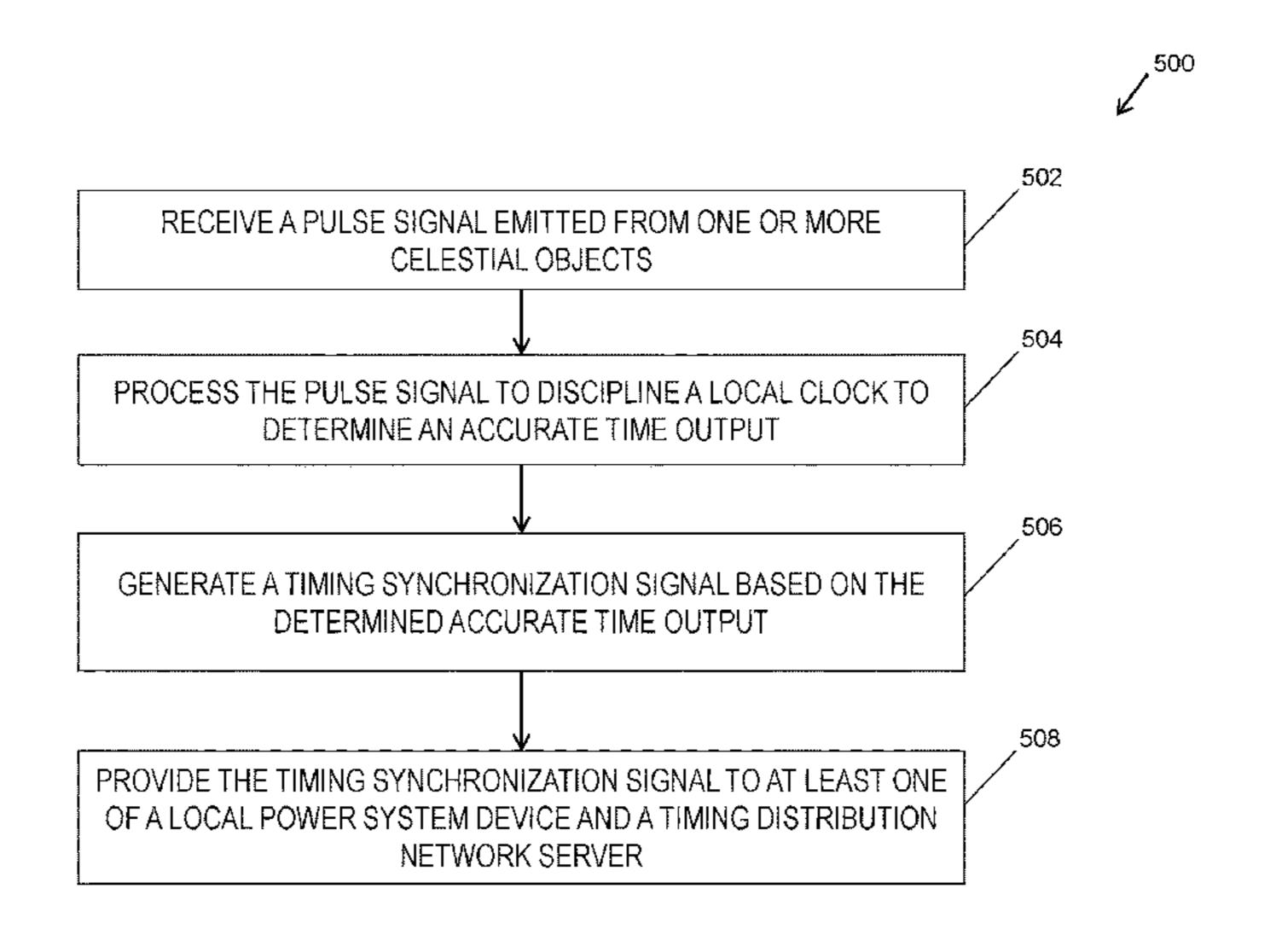
receiver device, a timing synchronization signal based on the determined accurate time output. The method further includes providing, by the pulsar signal receiver device, the timing synchronization signal to at least one of a local power system device and a timing distribution network server.
