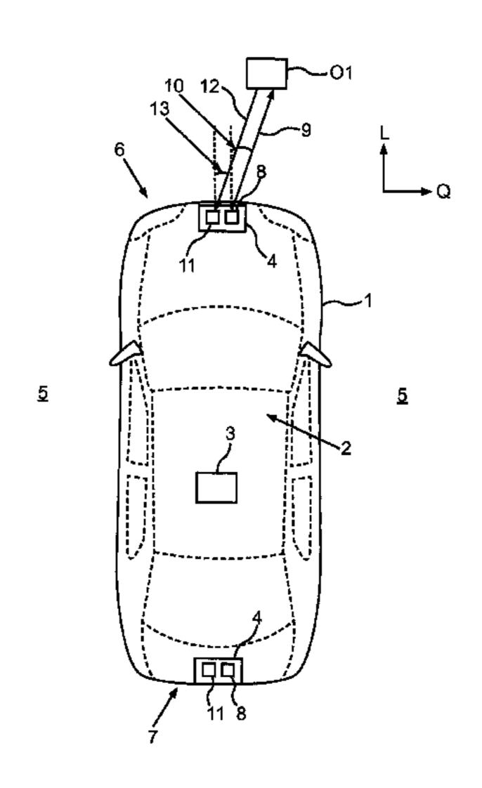
(5) is incident on the receiving unit (11), wherein the receiving unit (11) is designed to detect a deviation (17) between the emission angle (10) of the light beam (9) and the reception angle (13) of the reflected part (12) of the light beam (9) corresponding to the emission angle (10). The invention additionally relates to a driver assistance system (2), a motor vehicle (1), and a method for detecting a distance (x1) of an object (O1) in a surrounding region (5) of a motor vehicle (1).
