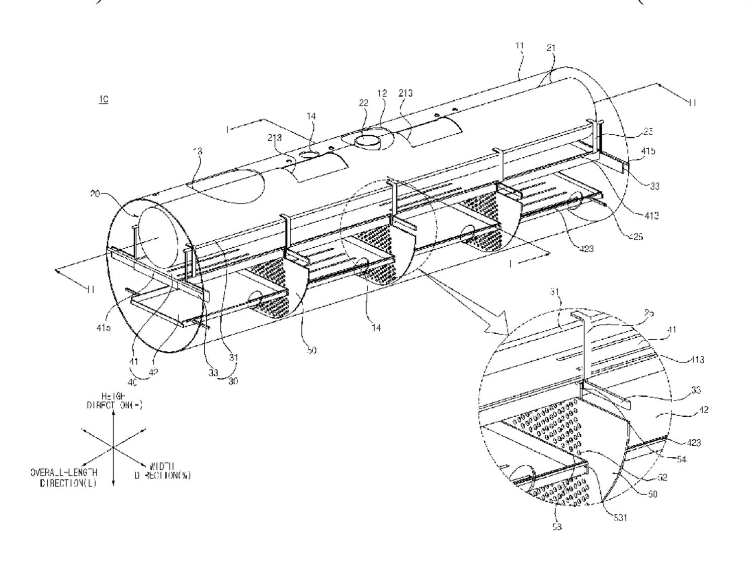
and supported by the support frames. Through the present disclosure, it is possible to keep the vapor-liquid separator horizontal and stable and achieve stable heat exchange performance.
