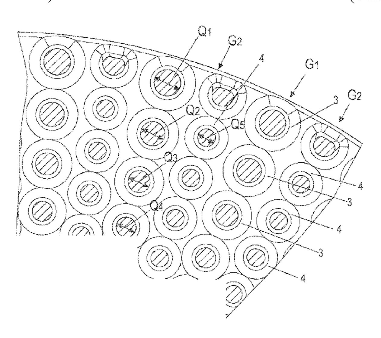
each other, where the cross-sections of a first subset of the ribs, embodied as supporting elements transmitting pressure forces, do not fall below a minimum cross-section, defined by the stability required in relation to the mechanical load during a brake process, and the cross-section of a second subset of the ribs, used to radiate thermal energy, falls below the minimum cross-section.
