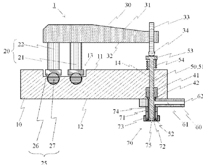
portion pressing the plunger downward, the plunger is pressed by the pressing portion, and the plunger is linearly reciprocated with rocking motion of the arm.
