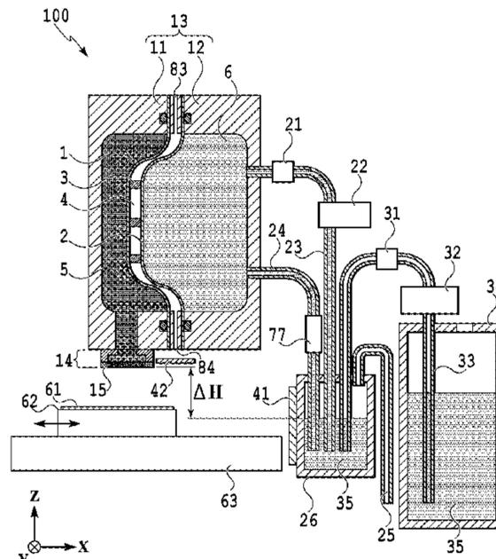
first storing space (5) and the second storing space (6) and the inter-film space (4) is detected with a liquid sensor (41), a flow speed sensor (77), and a liquid leakage sensor (42).
