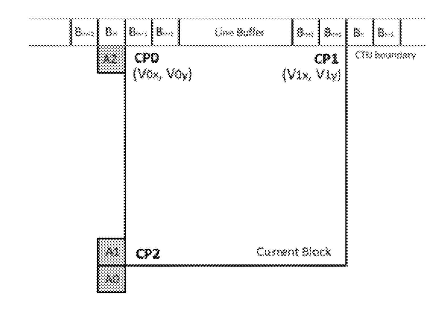
picture based on the motion information of the bottom locations in the neighboring block. Further, the processing circuitry reconstructs samples of the current block based on the affine model.
