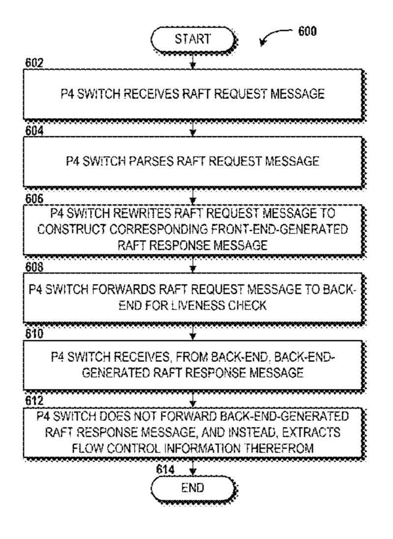
can maintain a complete state for responding to requests that cannot be fulfilled by the front-end. The requests can include read requests and/or write requests.
