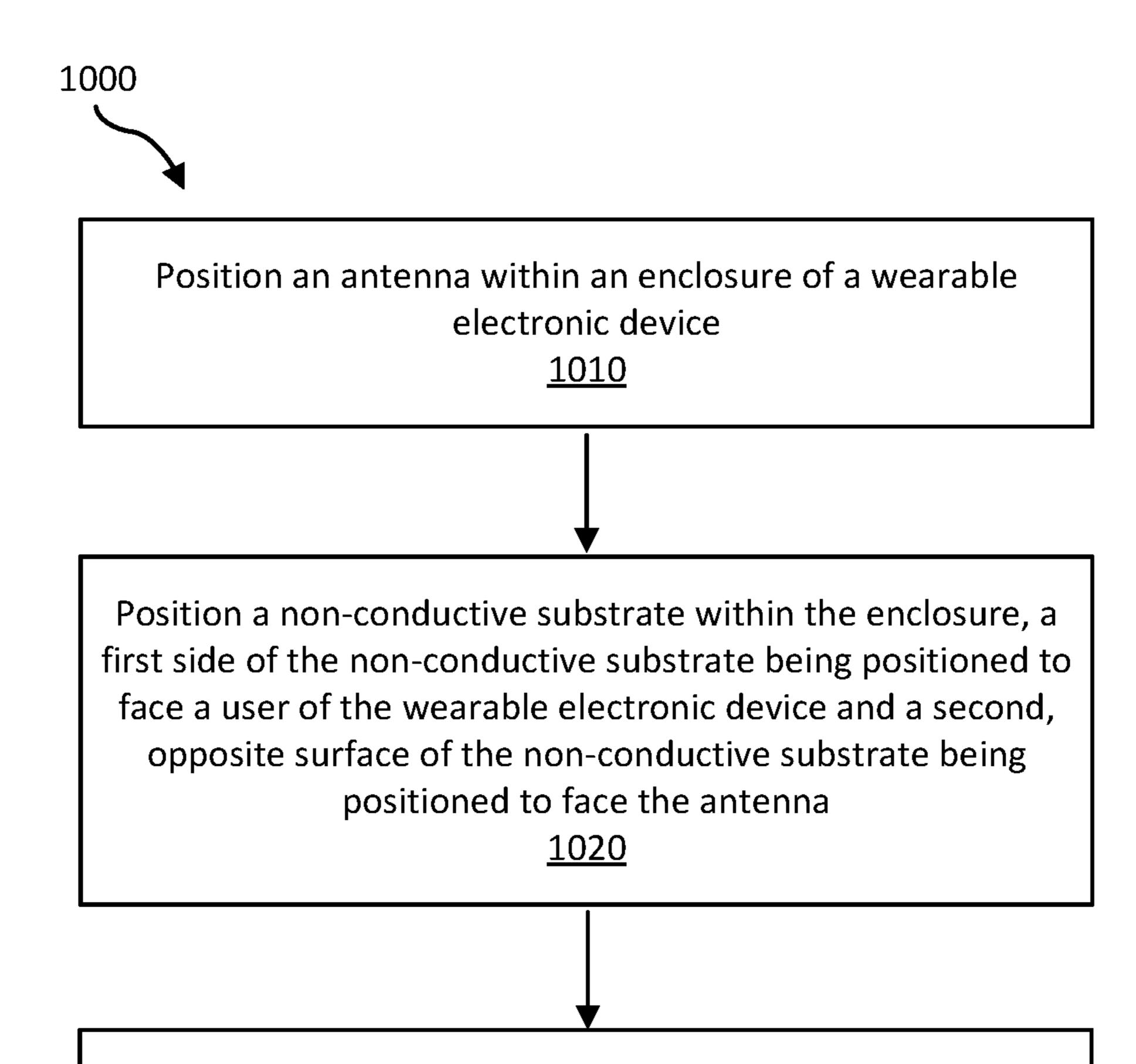
Apply a patterned conductive material on the second, opposite surface of the non-conductive substrate, wherein the patterned conductive material is shaped and configured to reduce electromagnetic signals radiated by the antenna in a direction towards the user of the wearable electronic device
