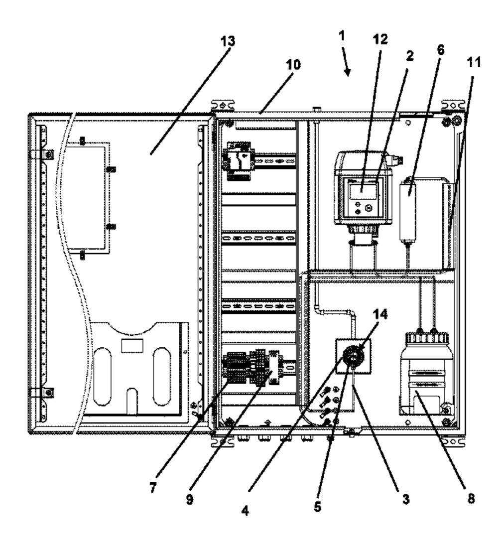
signal. A tap (4) removes compressed air and an actuator (5) changes a volume flow and/or mass flow of the compressed air, which volume flow and/or mass flow prevails in the measured air line. The actuator is inserted into the tap in a measuring mode and is removed from the tap in a compressed air removal mode.
