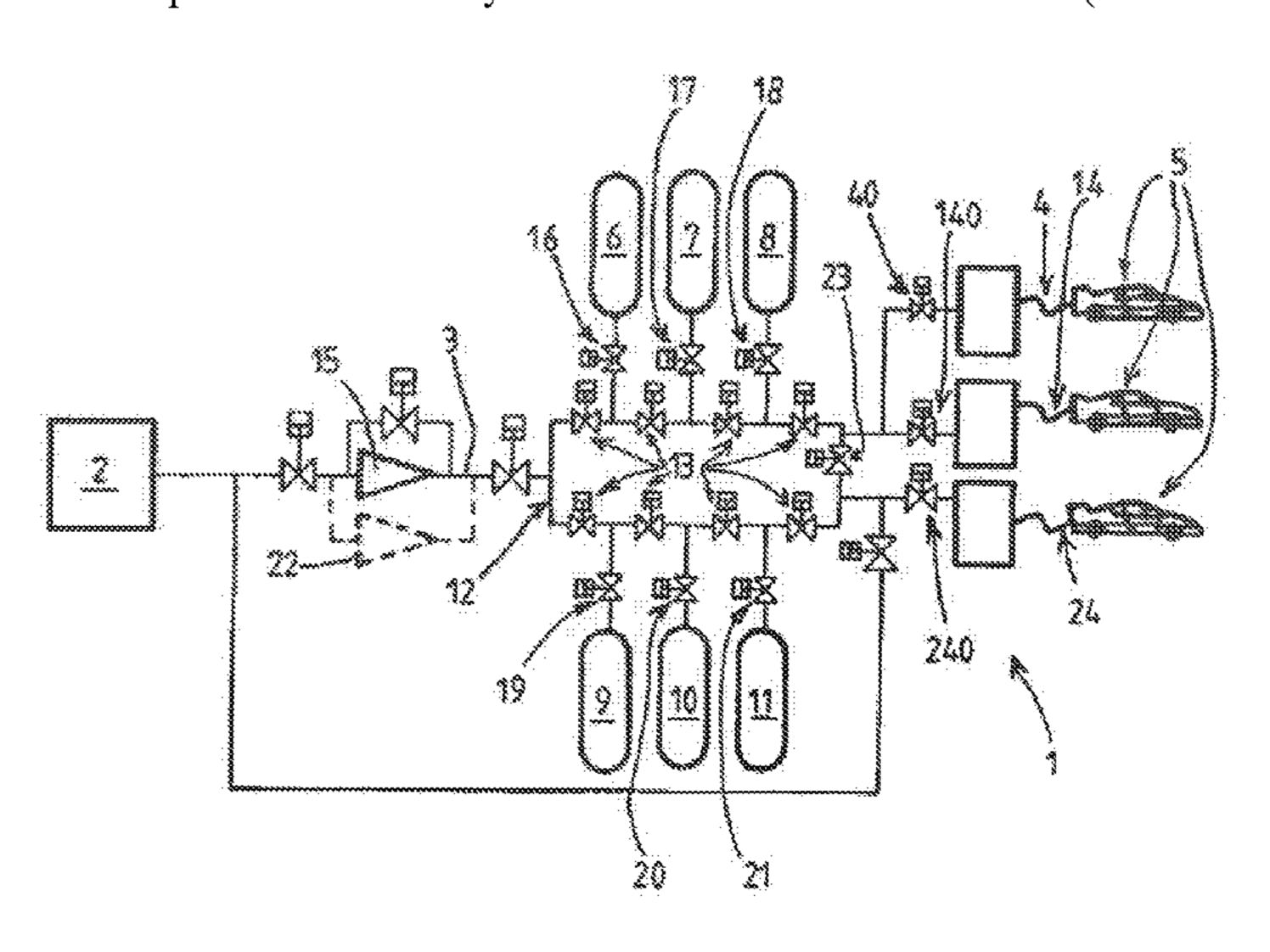
one second buffer storage container into fluidic communication, via the loop, with a second downstream end and/or to bring two separate buffer storage containers into fluidic communication.
