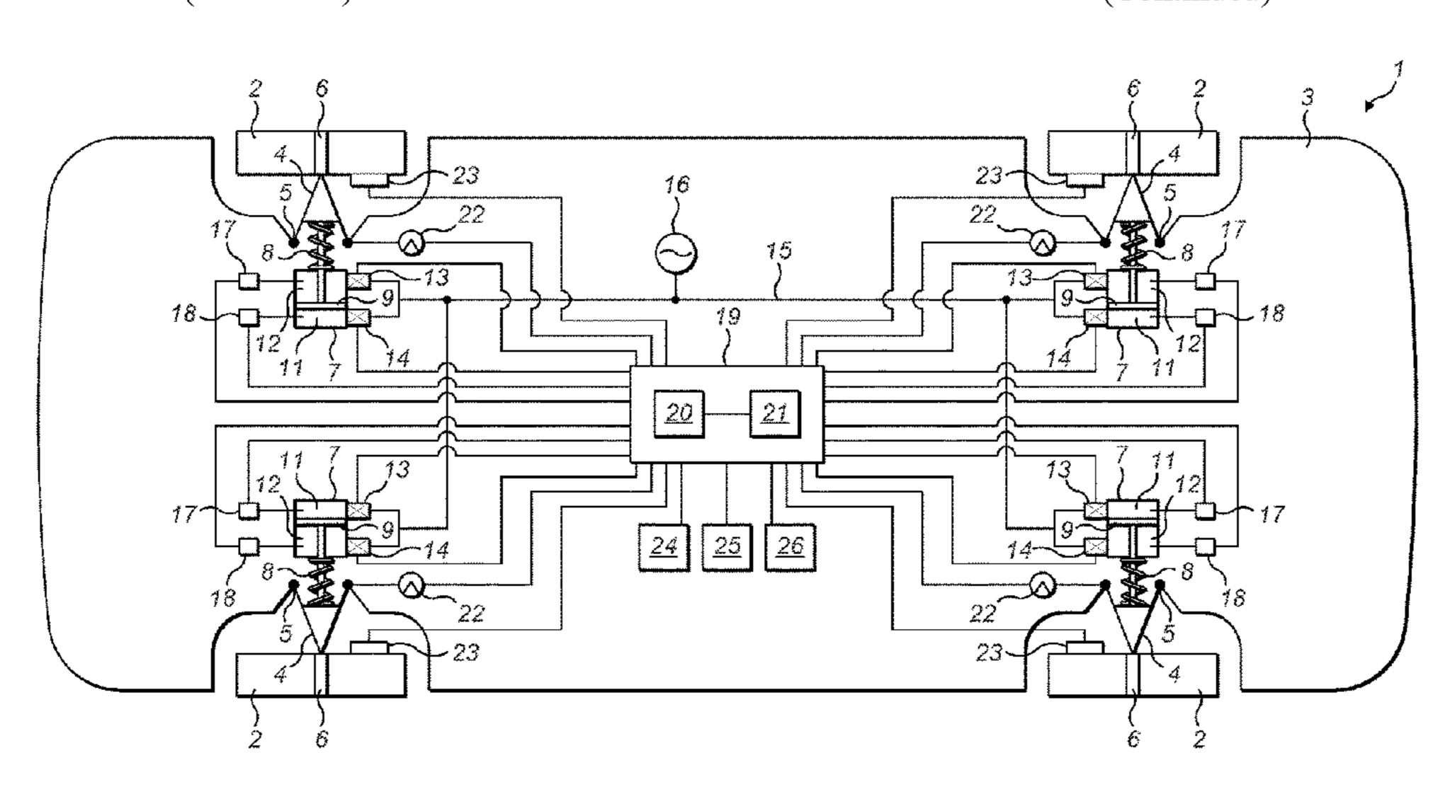
generate respective damper reaction forces to act against the suspension linkage to control the motion of the wheel assembly towards a set position for the wheel assembly relative to the vehicle body, adjust the set position based on a change in the vehicle condition data, and calculate the set position based on variations in the vehicle condition data over time.
