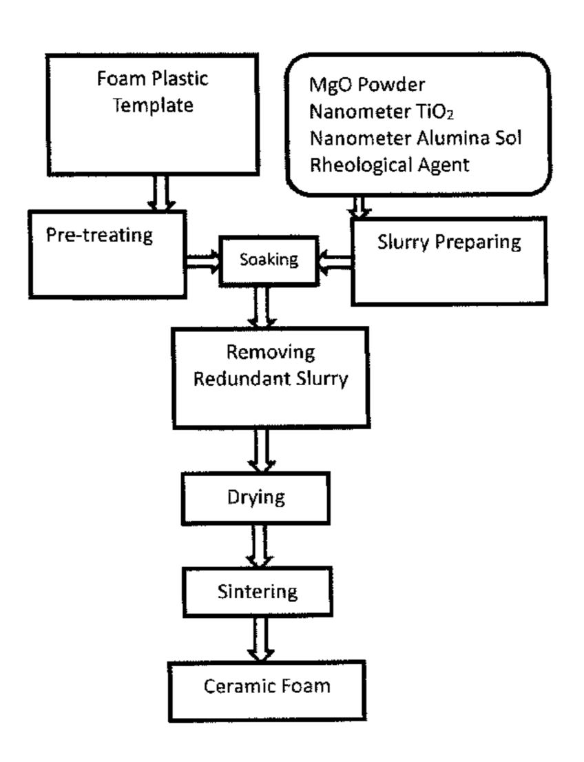
polyurethane foam plastic template to remove redundant slurry therein to make a biscuit, and drying the biscuit by heating it to 80° C.-120° C.; 3) putting the dried biscuit into a sintering furnace, elevating the temperature to 1400° C.-1600° C. and performing a high temperature sintering, cooling to the room temperature with the furnace to obtain the magnesium oxide-based ceramic foam filter.
