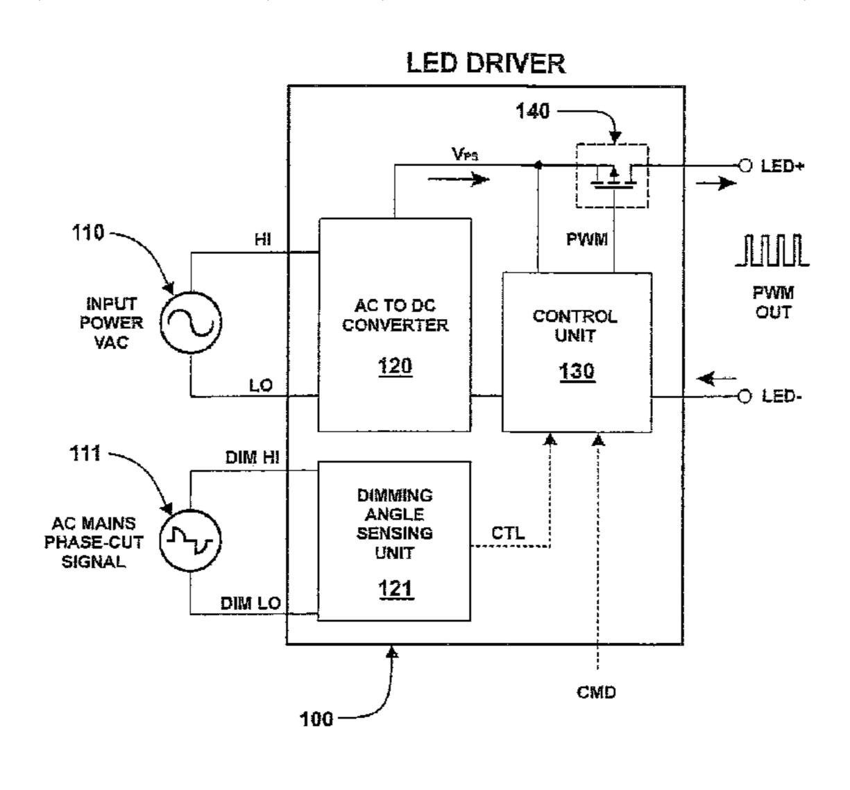
the control unit in order to connect or disconnect the DC power from the AC to DC converter.
